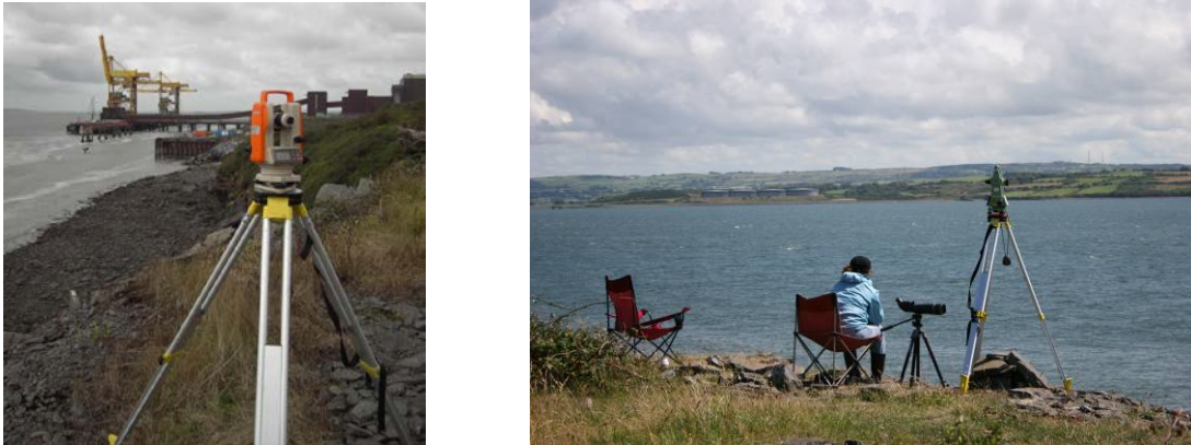
Figure 4.1 and 4.2: Theodolite set up with the reference point in the background (jetty at Moneypoint Power Station) and observer-based tracking
