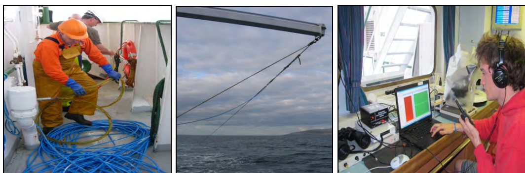
Figure 3.5: Towed hydrophone deployment and real-time monitoring
