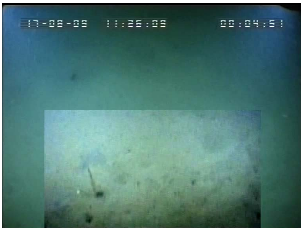
Figure 6.3. A frame grab from drop frame footage with Llyn video enhancement applied to the lower central part of the image, demonstrating the improved contrast, clarity and exposure. Under normal circumstances the enhancement would be applied to the whole of the frame.
