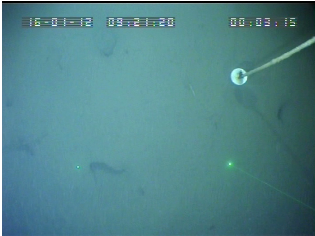
Figure 6.2. A frame grab from drop frame footage illustrating the location and effect of the lasers to provide a fixed field of view.
