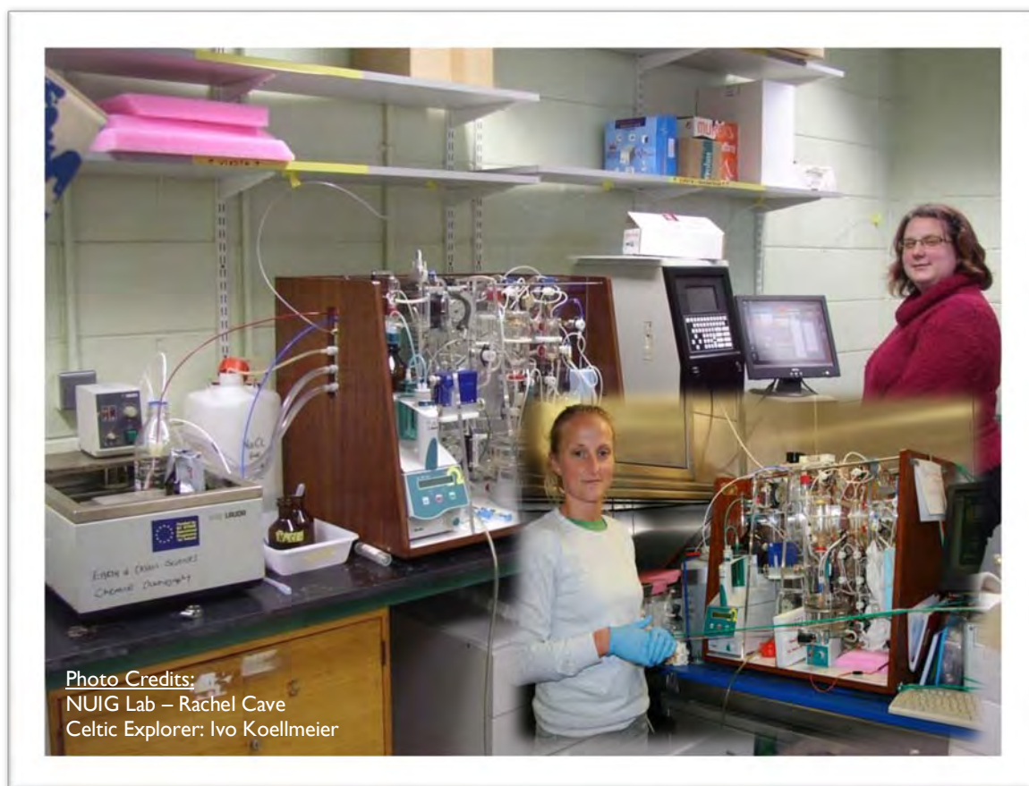
Figure 2.1: The VINDTA-3C (main picture, centre) with UIC coulometer (right) and water bath (left) for maintaining sample temperature at 25°C, in the lab at NUI Galway. Inset – the VINDTA installed in the chemistry lab on Celtic Explorer.
