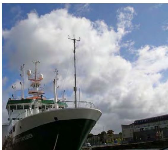
Figure 1.5: The R.V. Celtic Explorer. The \text{CO}_2 flux mast is seen at the front of the bow.
