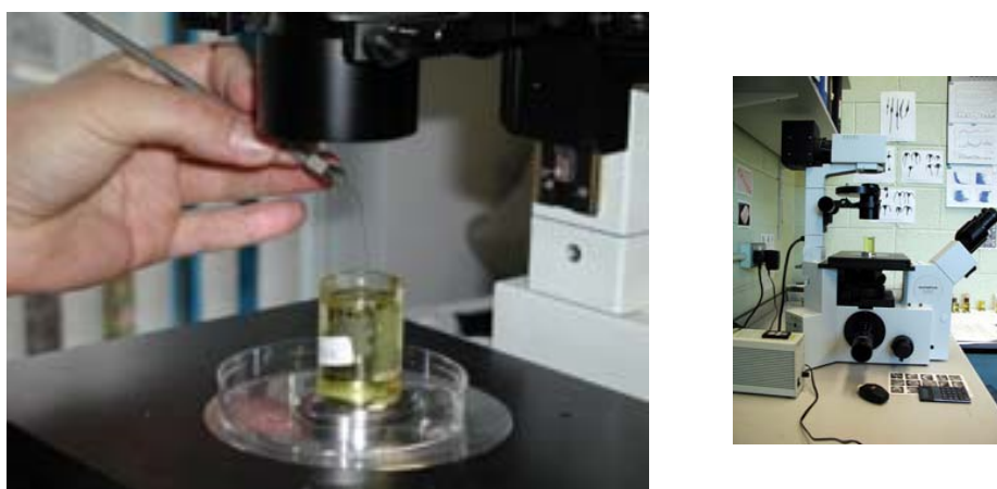
Figure 8. Picture of an inverted light microscope. The analyst is using an acupuncture needle to manipulate phytoplankton in order to help with the identification process.
