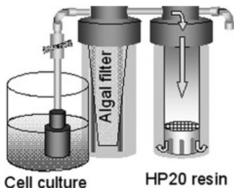
Figure 1. System for collection of YTXs from the P. reticulatum culture: Pump, filter and column with HP20-resin.
