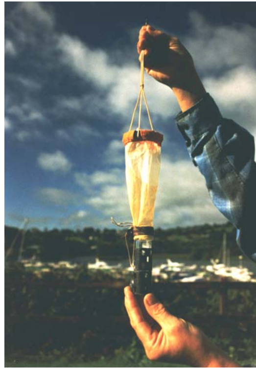
Plate 2. Plankton net used to catch zebra mussel larvae.
