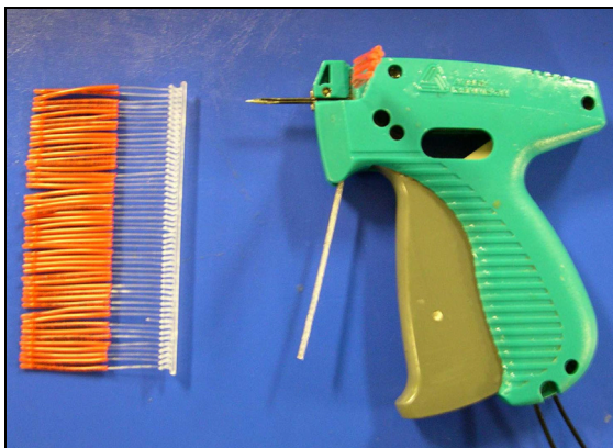
Figure 9. Avery Denison Tagfast III tag applicator and tags.
