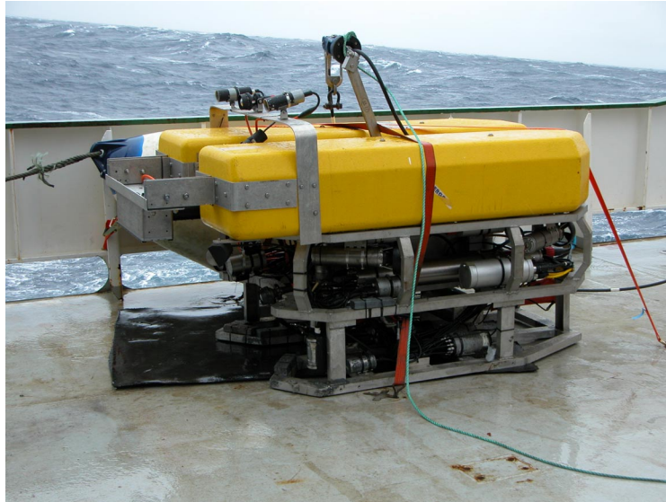
Figure 5. ROV Aglantha as used to record digital footage and high-resolution multibeam data on the sea floor.
