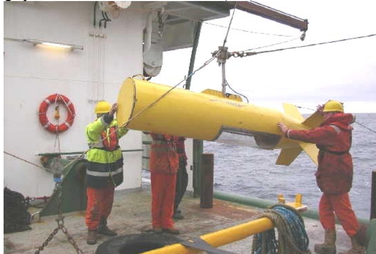
Figure 3. NIWA’s deep towbody used to acquire acoustic data on fish distribution around underwater features. Note: the transducer emits and receives echo through the perspex window on the lower surface of body.
