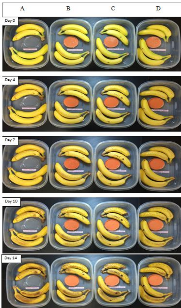
Figure 60 Banana test of peach juice-induced GCoU plate cells of R. rhodochrous DAP 96253. A. control; B. GCoU plate; C. GCoU plate with peach juice 1; D. GCoU plate with peach juice 2.
