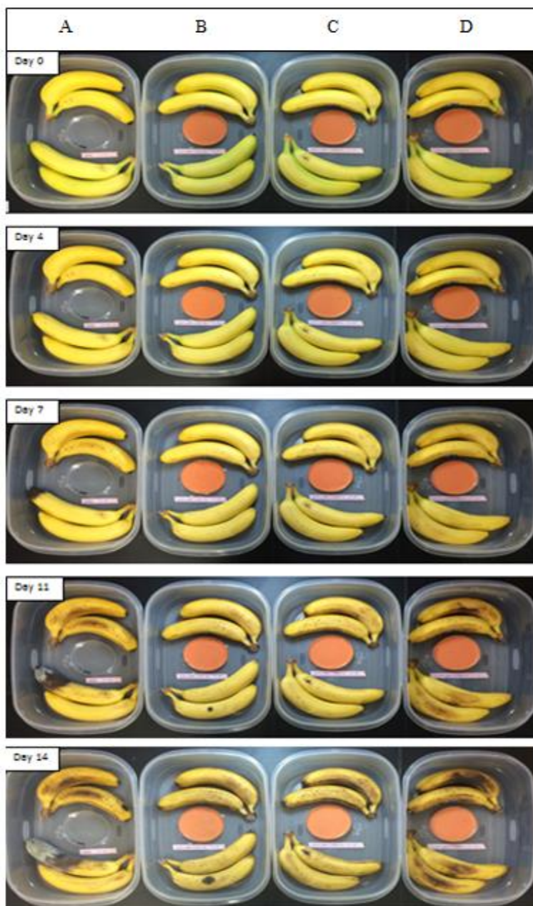
Figure 42 Banana test of ethylene and propylene-induced GCoU plate cells of R. rhodochrous DAP 96253. A. control; B. GCoU plate; C. GCoU plate with 100 ppm ethylene; D. GCoU plate with 100 ppm propylene.
