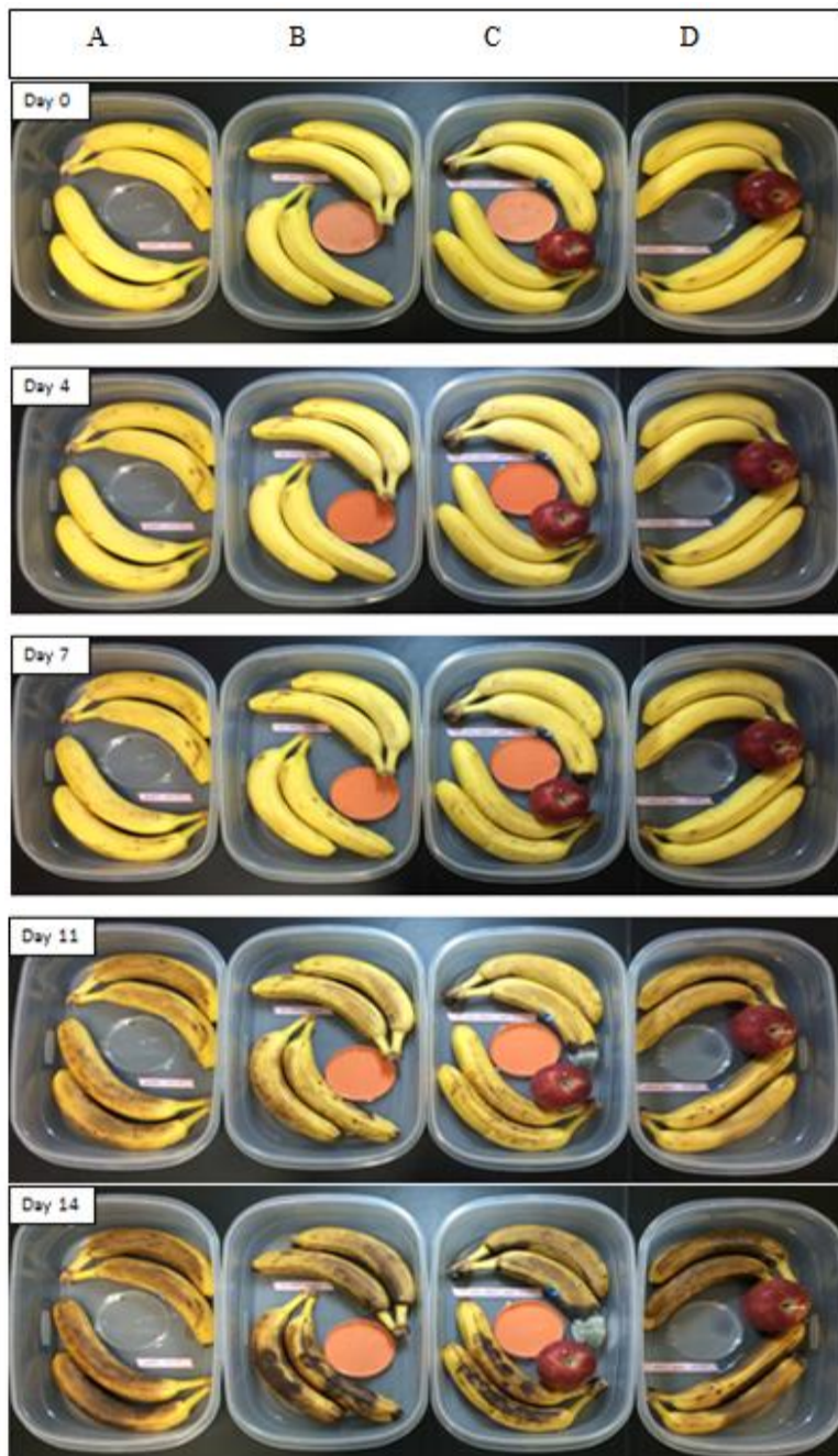
Figure 51 Banana test of organic apple-coordinated GU plate cells of R. rhodochrous DAP 96253. A. control; B. GU plate; C. GU plate with an organic apple; D. an organic apple.
