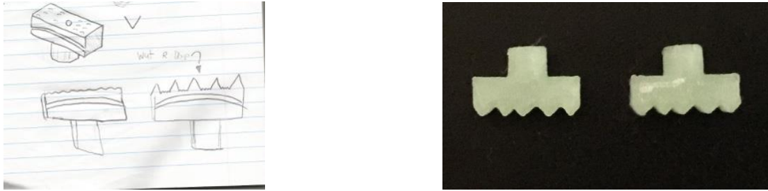
Figure 23. Student #7's Foot Design Draft and the Corresponding Printed Feet.
