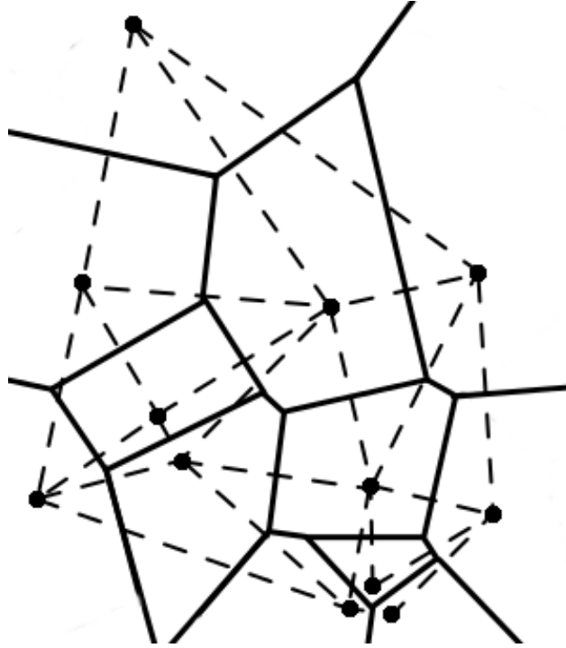
Figure 4.1: An example Voronoi diagram for objects on a 2-dimensional space. The black lines correspond to the borders of the Voronoi region, while the dashed lines correspond to the edges of the Delaunay Triangulation.
