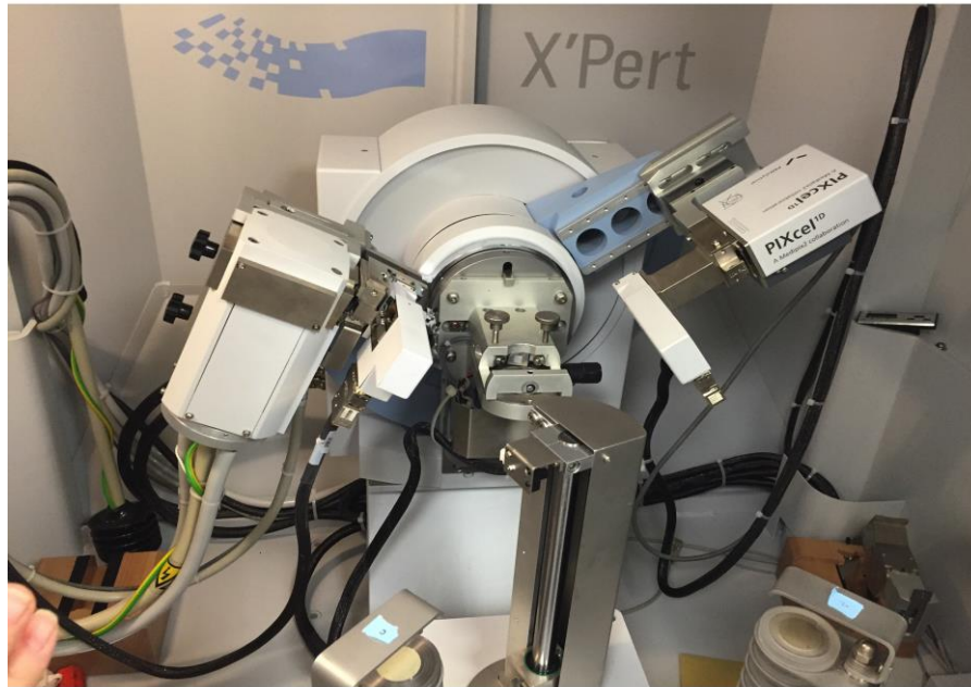
Figure 2-5 XRD PANalytical X'Pert PRO XRD
