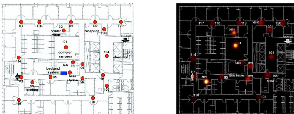
Figure 5.1 (a) Smart Office with sensors (b) Heat map based on sensor count in a week.
