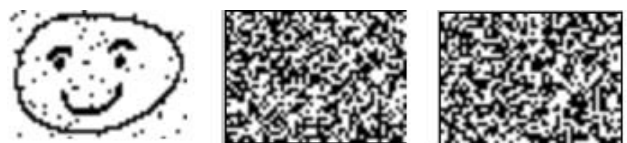
Figure 30. Happy face watermark images recovered from the Mountain (with salt and pepper noise): Haar, Coiflet 4, and Daubechies 32
