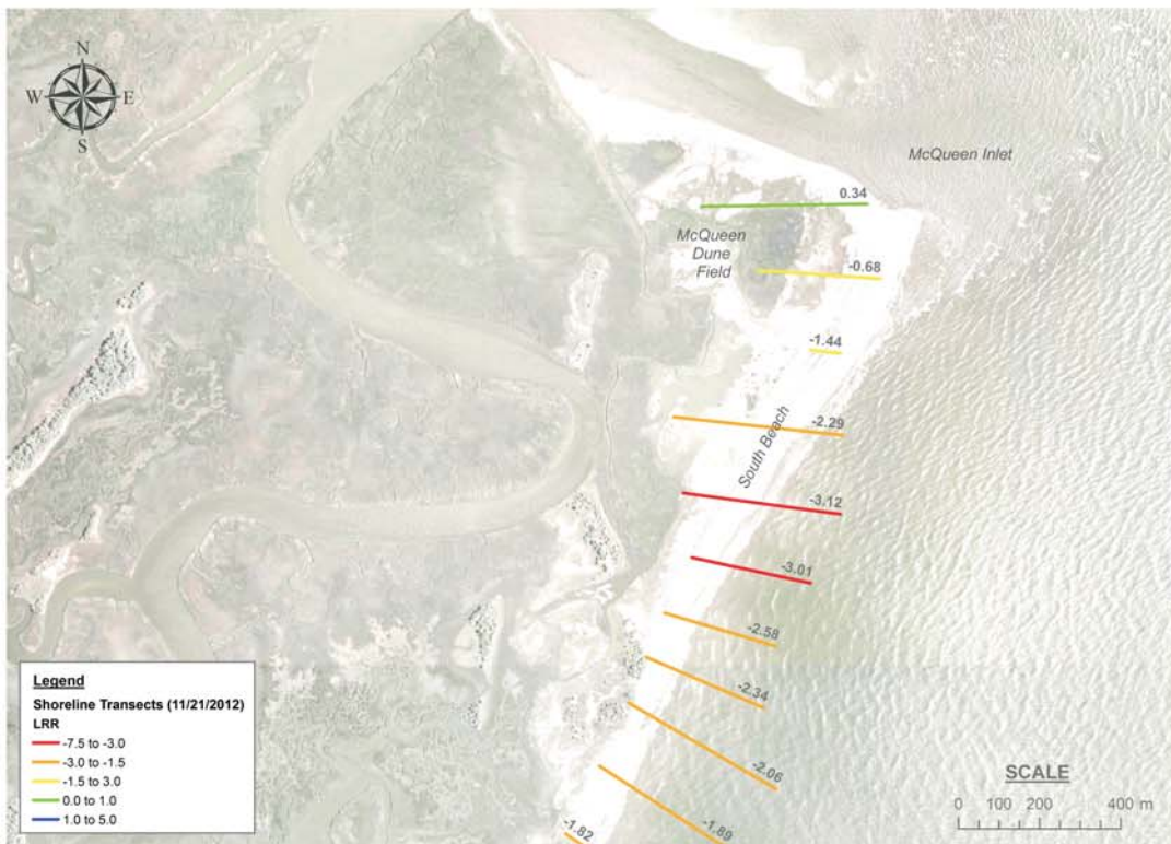
Figure A-6: Shoreline dynamics modeling results for the area located to the south of McQueen Inlet, results indicate net accretion immediately south of the inlet and appreciable rates of erosion to the south. Basemap image USDA NAIP (2009).
