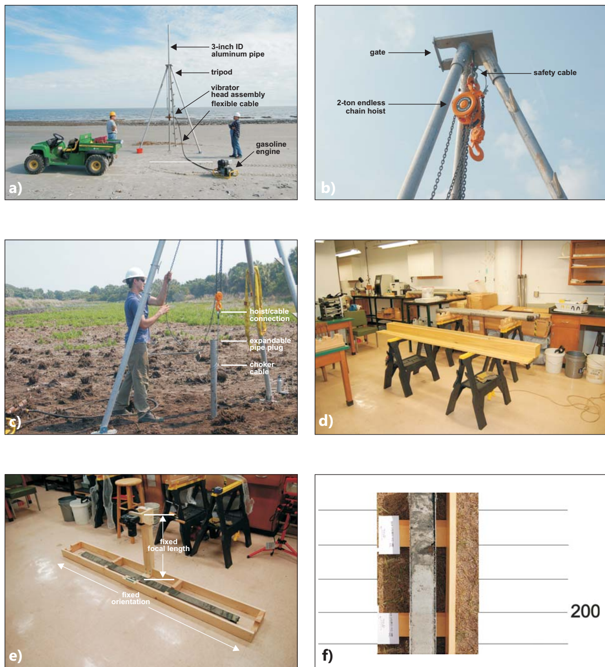
Figure 5-2: Equipment and methods in vibracoring. a) rig assembly consisting of the tripod, gasoline engine that powers the concrete vibrator via the flexible cable assembly and the vibrator head assembly that connects the vibrator to the 3-inch aluminum pipe, b) worker safety is promoted by utilizing a 2-ton endless chain hoist with safety braking, a safety cable for redundant measure, and a swinging gate to protect against the loss of control of the pipe during advancement/retrieval, c) retrieval of the core using an expanding pipe plug to create a vacuum, a choker cable to grab the pipe, and a grommet cable/hoist connection, d) cores are opened using a circular saw and the assistance of a fabricated wooden box to serve as a jig in guiding a true and safe cut, e) cores are photographed using a fabricated copy stand, and f) a high resolution photographic image is produced using multiple images and a photographic log is produced. Photographs by B. Meyer.
