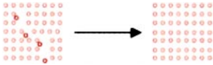
Fig. 9 Perfect is the condition where all atoms lined up on crystal lattice sites, there are no defects, and this is the lowest energy “state” for this set of atoms.
