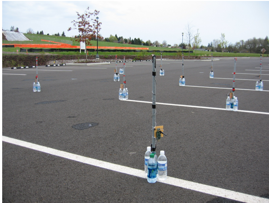
Figure 3.6 Outdoor experiment test-bed of 15 nodes synchronized by WWVB radio.
