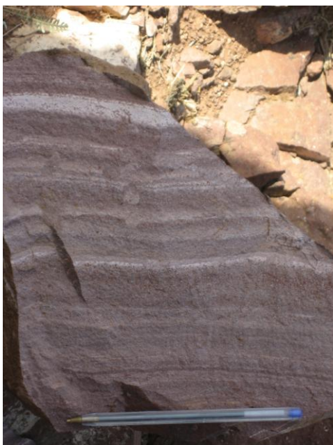
Figure 3.20. Red, crystal-lithic tuff. Pen provides scale.
