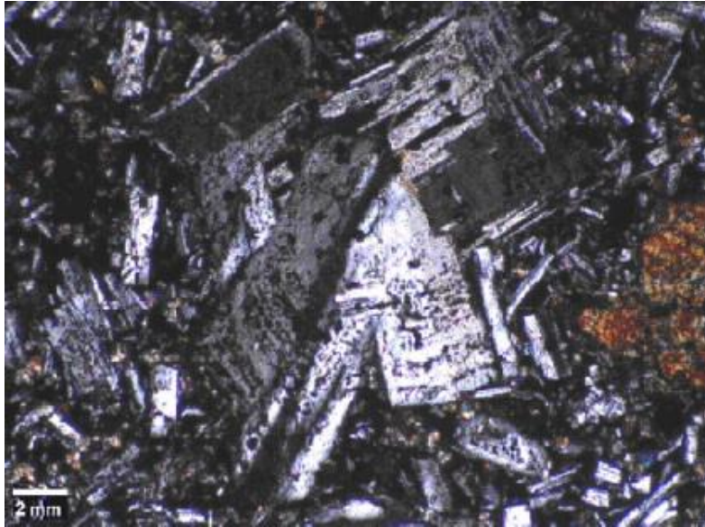
Figure 3.24. Photomicrograph showing twinned and zoned plagioclase (KM 30).
