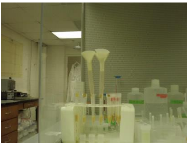
Figure 2.5. Primary (exchange) columns filled with resin (AG 50W-X8).
