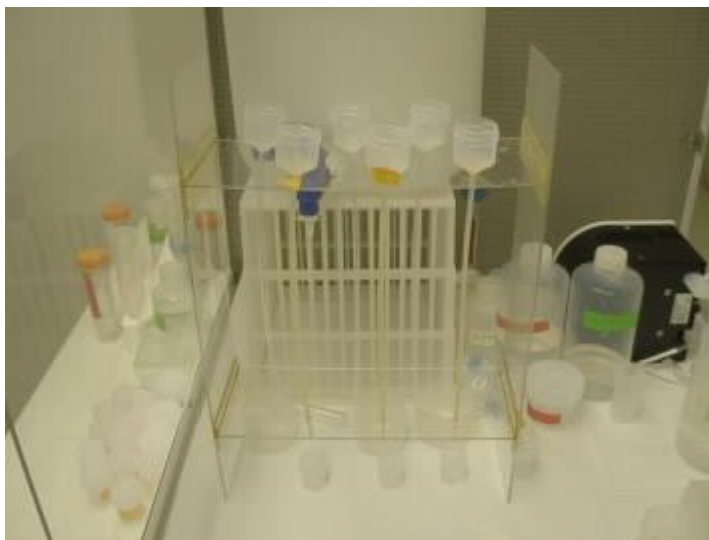
Figure 2.6. Secondary (exchange) columns or \alpha -HIBA. Secondary columns filled with resin (AG 50W-X4).
