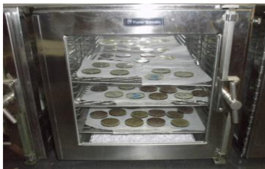
Figure 2.11. The desiccating cabinet containing the glass disks.
