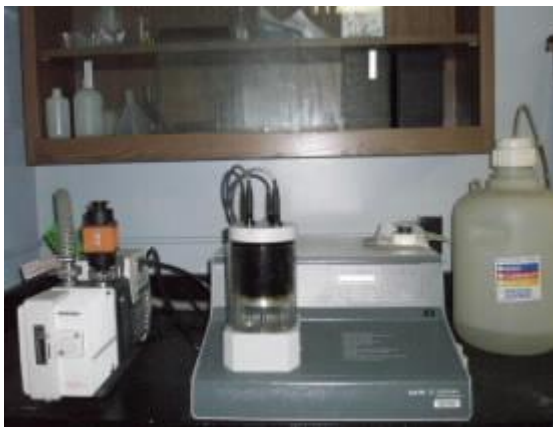
Figure 2.1. Vacuum turbo carbon coater.
