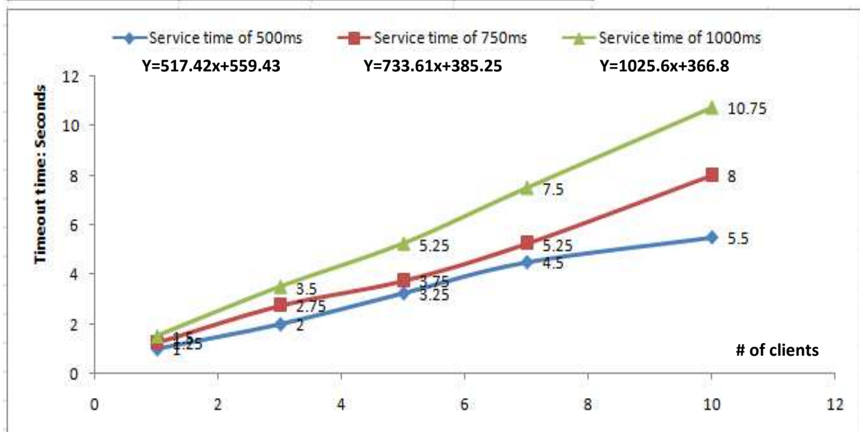
Figure 26. The increasing numbers of clients and service time on the server influence the timeout time linearly.
