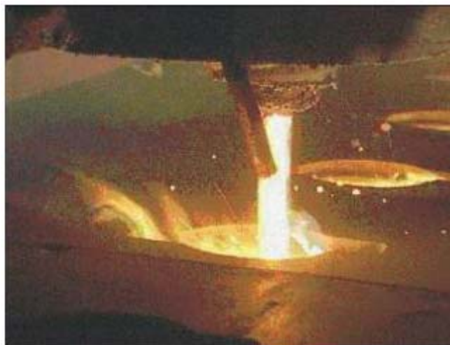
Figure 1.5: Pouring of Molten Metal [8]
