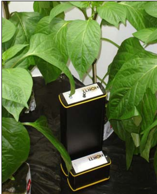
Figure 4.1: The HortiSpec can be connected wireless via Bluetooth to a distant computer. The computer can then be used to control the movement of screen filters in the greenhouse or to control special lamps. It was developed to measure the light intensity and spectral distribution in the visible and NIR range inside greenhouses.
