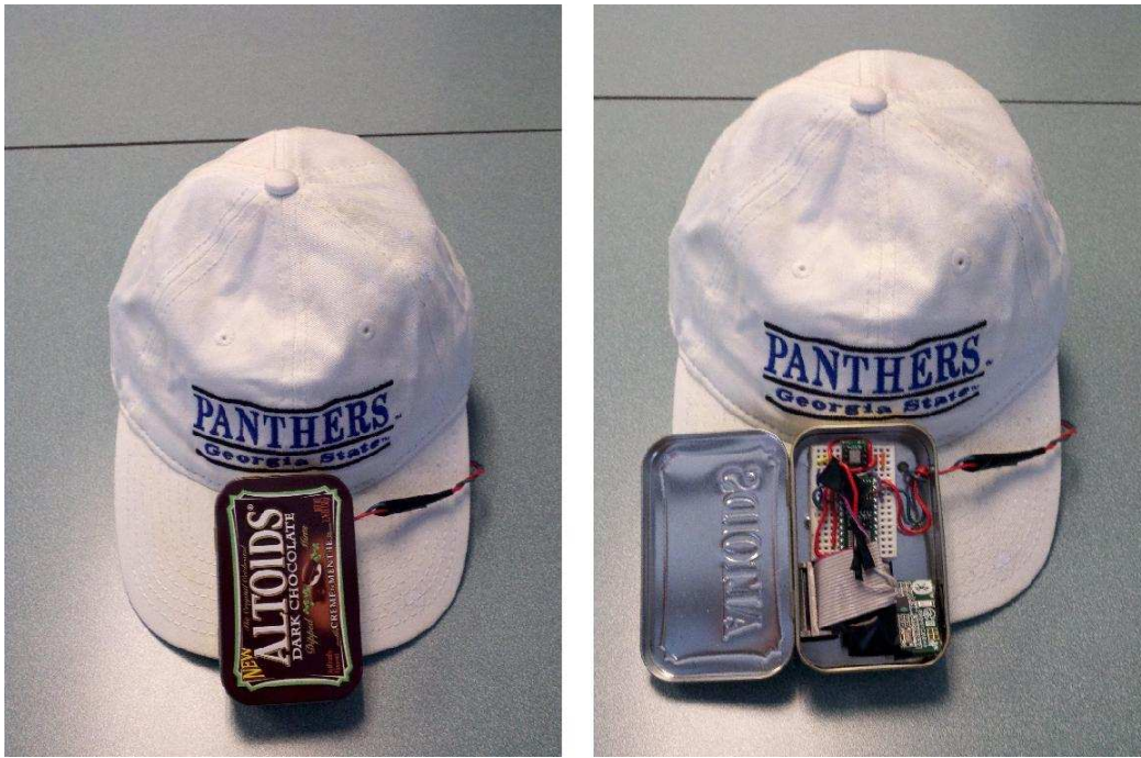
Figure 2.10. Head-tilt mouse embedded in baseball cap
