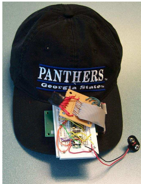
Figure 2.11. First version of head-tilt mouse embedded in baseball cap
