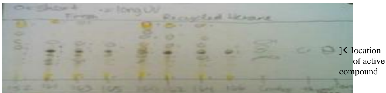
Figure 24: TLC results of graduated extraction of thyme leaves using recycled and non-recycled hexane.
