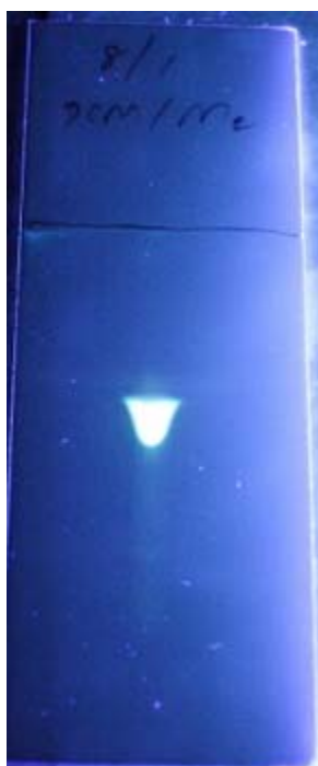
Figure 19: TLC plate of V-3. The solvent used to develop the plate is 8:1 DCM/methanol.
