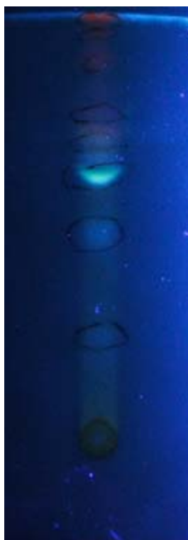
Figure 14: TLC plate of F-4. The solvent used to develop the plate is 10:1DCM/methanol.
