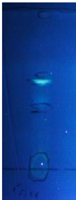
Figure 16: TLC plate of G-4 and G-5 combined. The solvent used to develop the plate is 8:1DCM/methanol.
