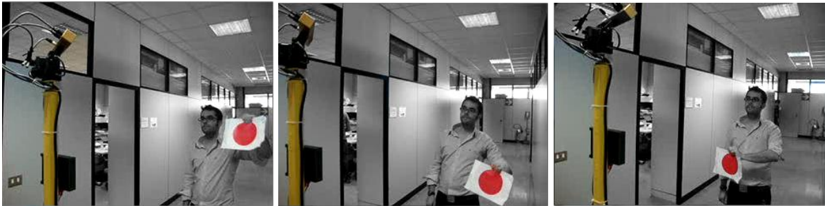
Fig. 24. Tracking the moving target in real-time
