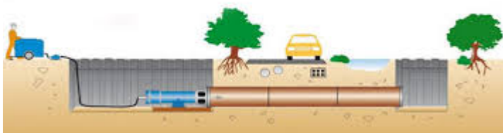
Imagen N°11: Pipe Ramming (Underground Brown, 2014)
