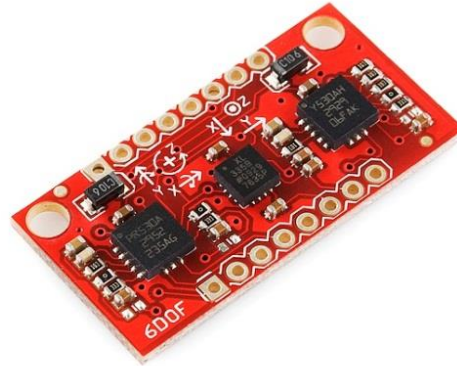
Figure 29. Inertial Measurement Unit.
