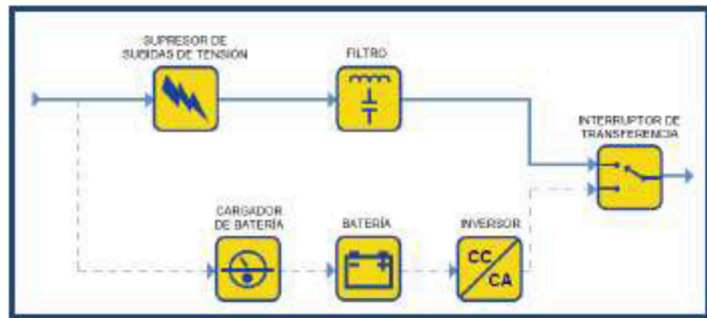
Figura 27. UPS off line o Standby.
