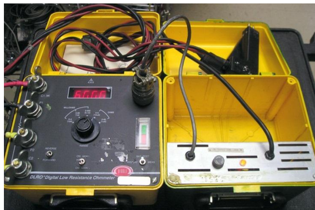
Figura No. 15. Óhmetro de baja resistencia – Biddle DLRO247000 Low Resistance Ohmmeter [23]
