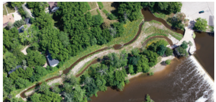
This aerial photo of the Mequon-Thiensville Dam shows an example of a nature-like fishway that flows to the side of the dam, allowing fish passage without removing the dam. Photo courtesy of Stantec.
