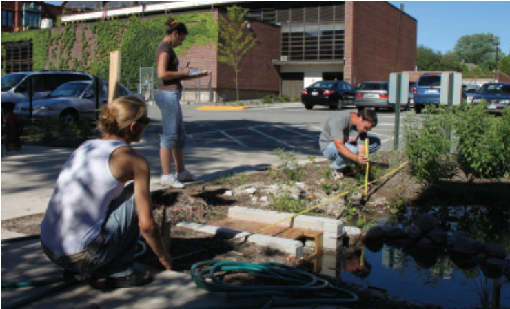
Three students determine the volume and contours of a swale in the spiral garden. Understanding the volume and other aspects of a swale allows engineers and landscape architects to calculate the positive impact the bioswale can have during a heavy rain event—helping to slow and absorb water as it flows through the depression. Photo courtesy of Jim Wasley.
