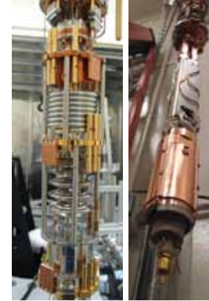
Above: Maintaining the STM's ultra-low temperatures: the cryogenics and microscope head before insertion into the cryostat.
