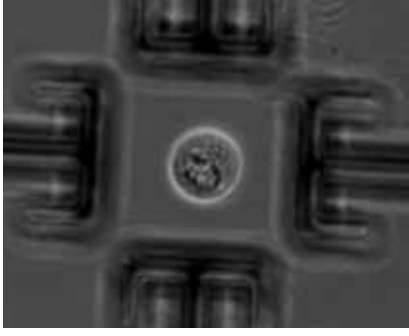
Above: Time-sequenced high-frequency voltage applied to the eight microelectrodes exerts dielectrophoretic forces, rotating the cell they surround.
