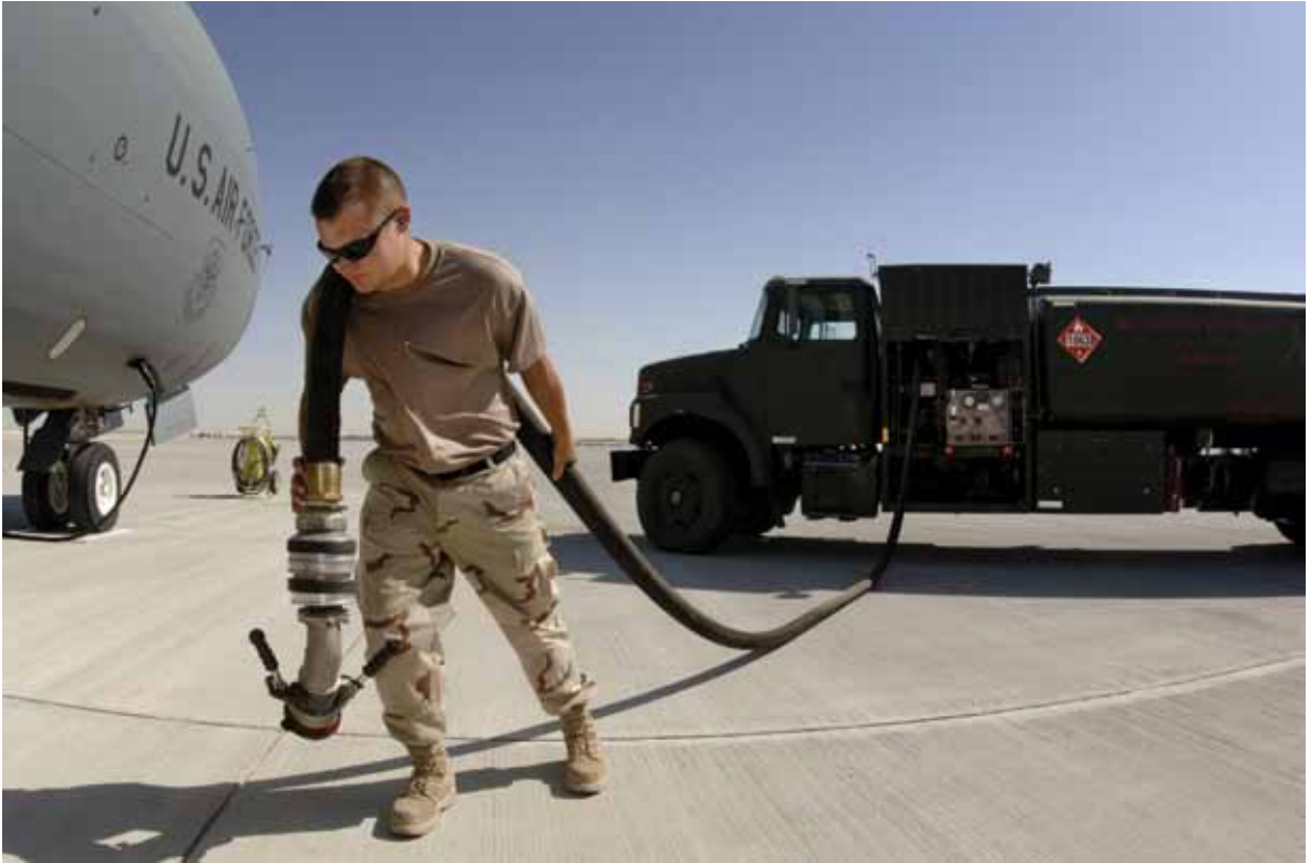
U.S. AIR FORCE AIRMAN MARK HEITKAMP PULLS A FUEL SERVICE HOSE FROM AN R-11 FUEL TRUCK IN PREPARATION FOR REFUELING A KC-135 STRATOTANKER AIRCRAFT WITH JP-8 FUEL AT AN AIR BASE IN SOUTHWEST ASIA ON MAY 31, 2006.
