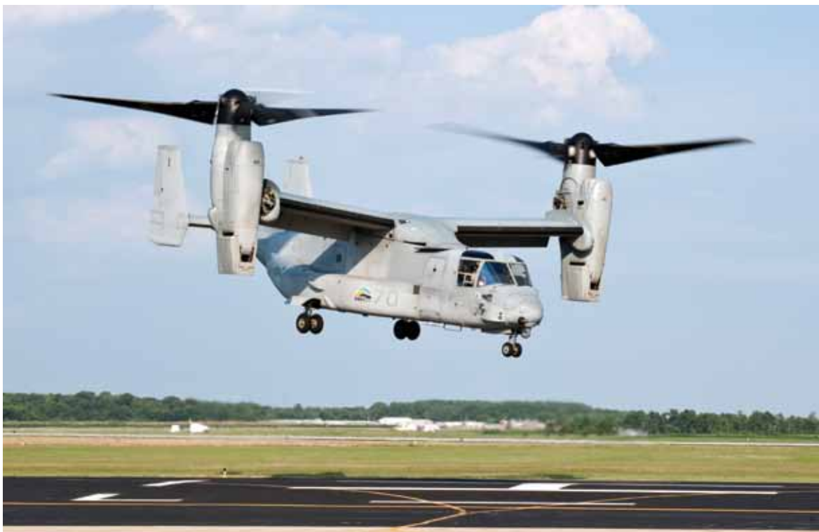
A U.S. MARINE CORPS MV-22 OSPREY LIFTS OFF FROM NAVAL AIR STATION PATUXENT RIVER, MD., DURING A SUCCESSFUL BIOFUEL TEST FLIGHT. THE TILT-ROTOR AIRCRAFT FLEW AT ALTITUDES OF UP TO 25,000 FEET ON A 50-50 BLEND OF CAMELINA BASED BIOFUEL AND STANDARD PETROLEUM BASED JP-5 FUEL.
