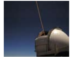
Keck II uses a laser to create an artificial guide star for adaptive optics.
