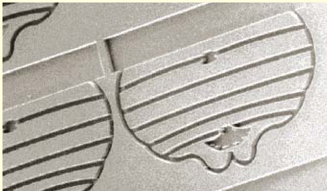
MEMBRANE PATTERN ETCHED INTO SILICON SUBSTRATE
