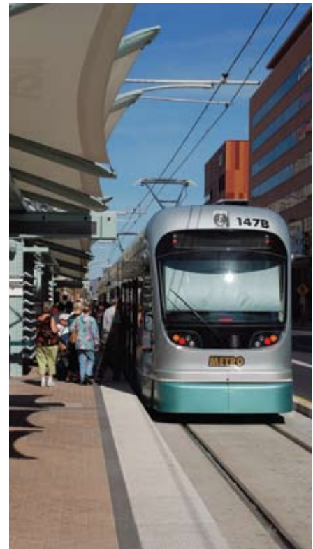
The new light-rail line in Phoenix, Arizona, can accommodate up to 12,000 passengers per hour, the same as a six-lane highway. (Valley METRO)
