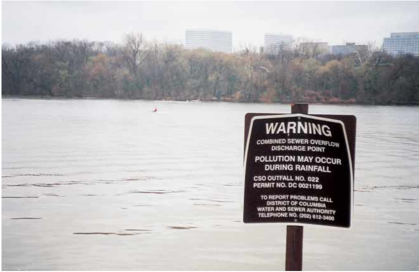
The city's combined sewer system was designed to overflow stormwater and raw sewage at 58 different discharge points throughout the three rivers of the District of Columbia—including here on the Potomac River, between the Kennedy Center for Performing Arts and the Georgetown waterfront.
