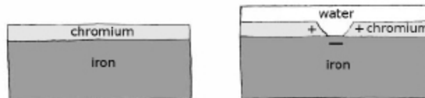
cathodic protection - chromium plating on iron
