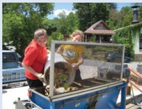
Tory Selz and Emily Holzer empty food waste into the mixer of Warren Wilson's in-vessel GreenDrum composter.
