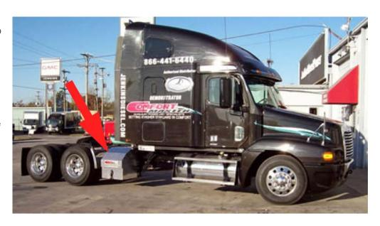
A Comfort Master APU attached to the underside of the truck between the cab and wheel base. (Source: www.comfortmaster.com)
