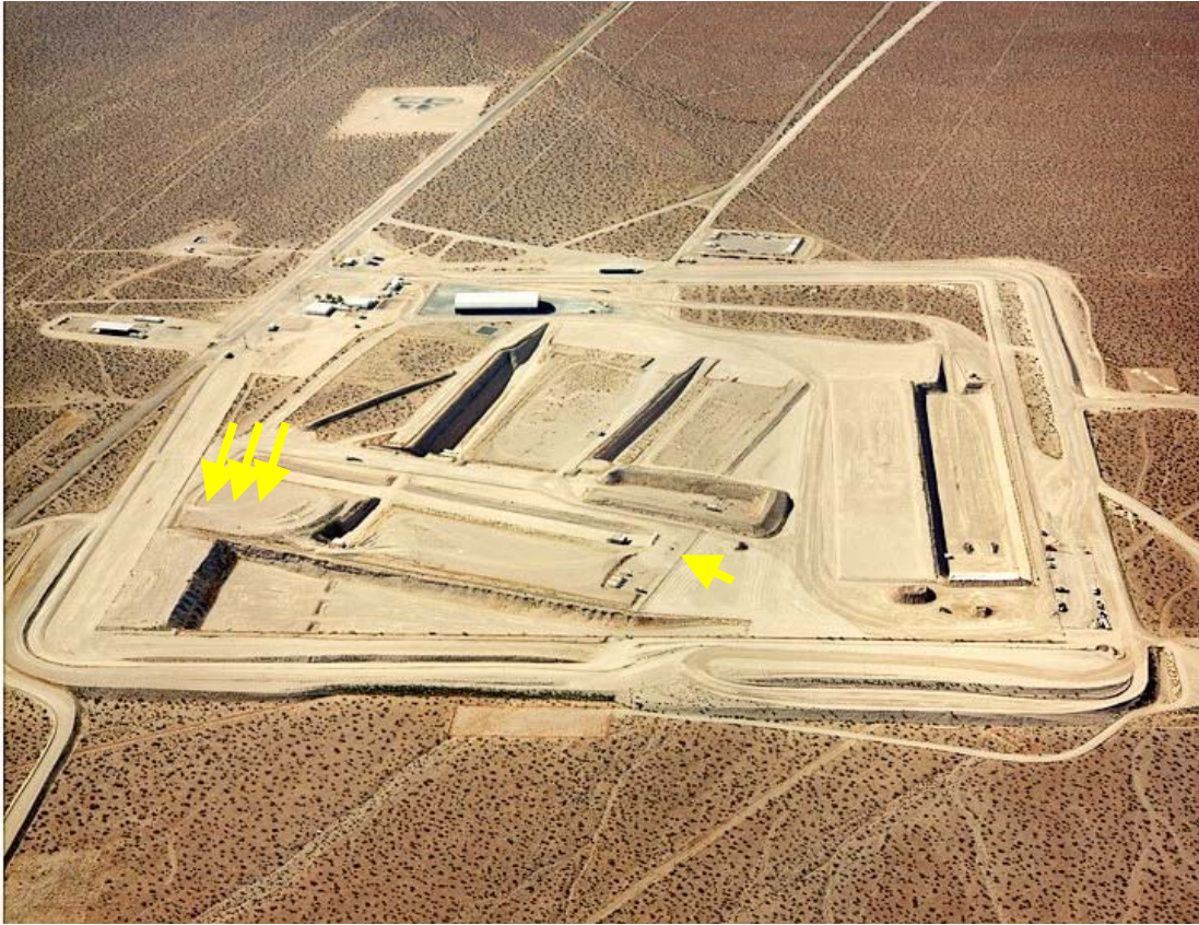
Figure 2. Aerial view of the Area 5 RWMS showing the pit and trench configurations used for disposal of LLW. The yellow arrows mark the approximate locations of the four TRU GCD boreholes.
