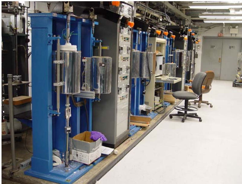
Fig. 25: Ten lever arm creep machines refurbished for testing CMS Alloy 617 and Alloy 230 in air environment
