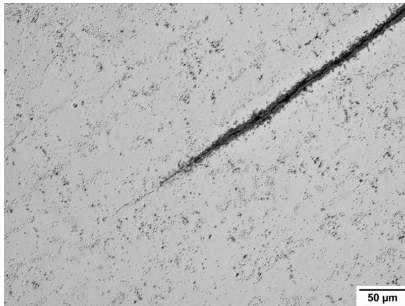
Fig. 47: Close view of tip of large crack shown in Fig. 46
