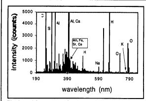
Fig. 3. LIBS spectrum of 10% soil in ice. The spectrum is the average of 40 shots.
