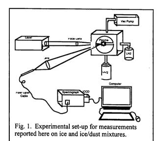
constant flow of CO<sub>2</sub> gas was maintained through the chamber.
