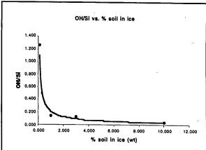
Fig. 4. Determination of the relative amount of soil in ice using the OH/Si ratio.
