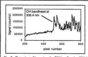
Fig. 2. Detection of ice using the OH bandhead at 306.4 nm.
