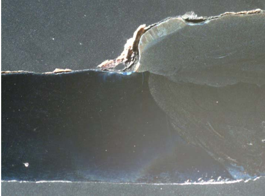
Modified 800H Adjacent to Weld "Z"
