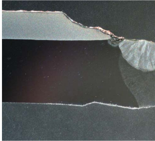
Figure 13: Weld Profile Through Clad Tube Sample Incoclad 671 Adjacent to Weld "P" (at 1203 F) in Section C
