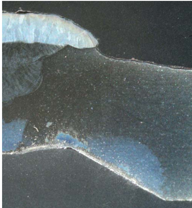
(b) HR 120 Adjacent to Weld "V"
