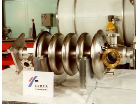
Fig. 2. One of four 5-cell 700-MHz \beta=0.64 niobium elliptical accelerating cavities built for LANL by CERCA.
