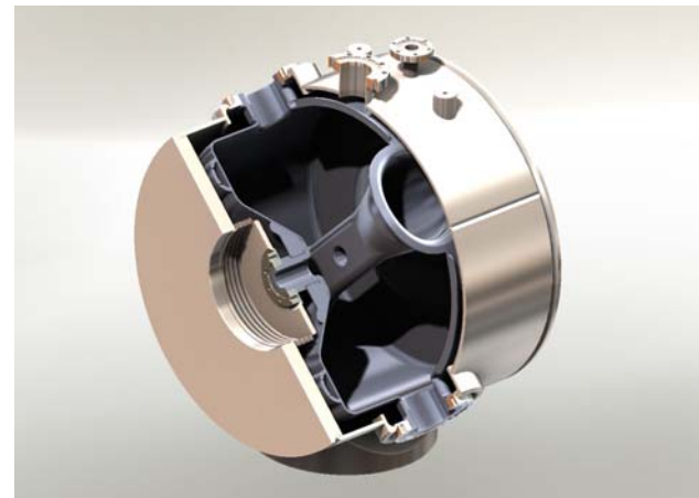
Figure 6 : Cut out view of the SSR1 cavity inside the helium vessel.
