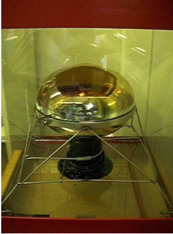
Figure 4.8: A typical phototube used in the MiniBooNE detector: an 8 inch Hamamatsu R1408 mounted on its wire frame.
