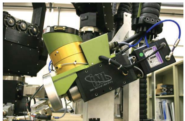
Figure 4: Weld dressing end effector used for wire brushing and grinding.
