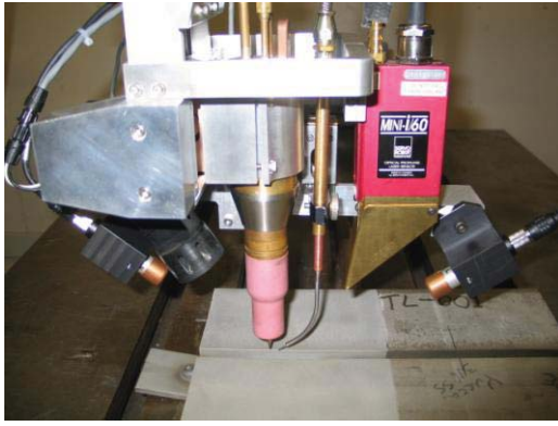
Figure 2: Welding end effector showing air cooled weld torch, weld viewing cameras, and laser line scanning sensor for visual weld inspection.
