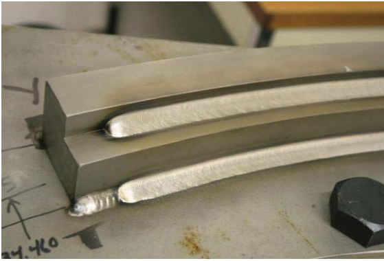
Figure 5: A pair of two pass fillet welds are shown in a 316 stainless steel coupon. This coupon simulates seal welds in a particular vessel under development.
