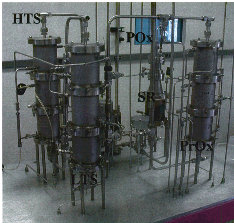
Figure 1. Fuel processor system showing the stages for Partial Oxidation (POx)/Steam reforming, High Temperature Shift (HTS), Low Temperature Shift (LTS) and Preferential Oxidation (PrOx).
