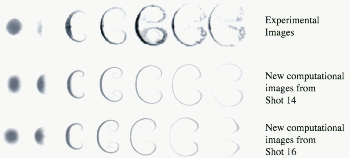
Fig. 16. A graphical comparison of shock tube experimental images to the corresponding SAGE simulations. The images show a progression of dynamical shapes as the evolution of the initial cylinder moves downstream. Also included in Zoldi's work is a good comparison of code results for velocity distributions to those obtained from the experiment.
