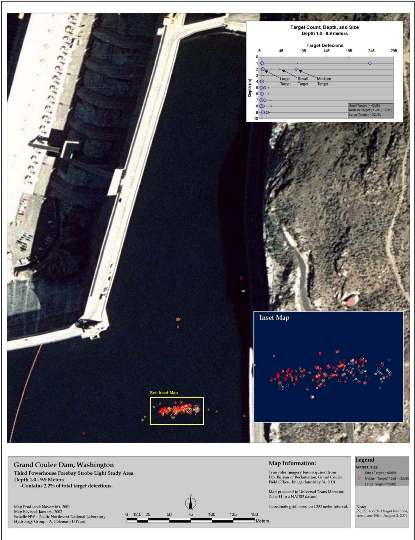
Figure B.4. Location of Targets Within 10 m of the Surface Detected by the Mobile Hydroacoustic Surveys in 2001. Three size-groups of targets are indicated based on target strength (dB).
