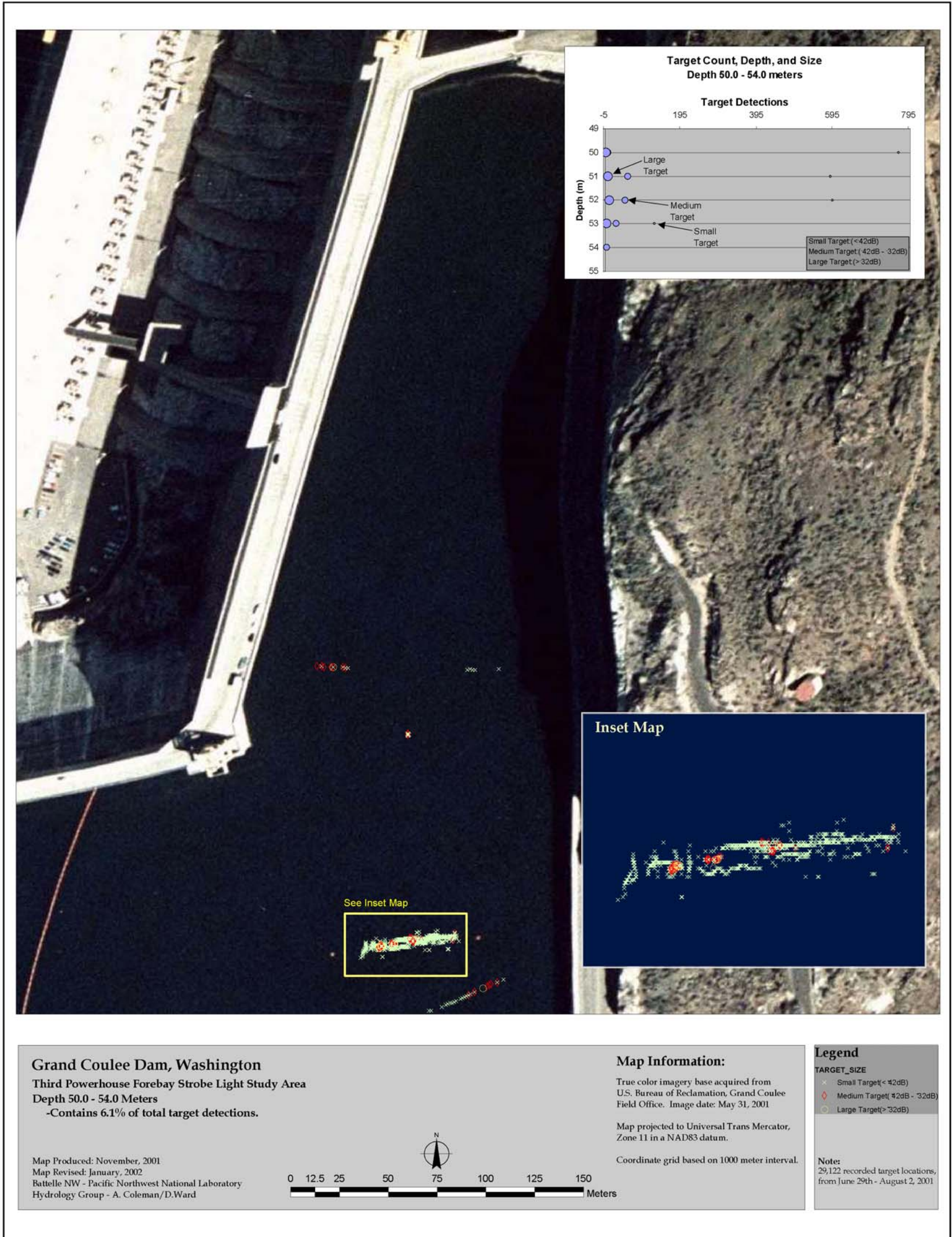
Figure B.9. Location of Targets Between 50-54 m from the Surface Detected by the Mobile Hydroacoustic Surveys in 2001. Three size-groups of targets are indicated based on target strength (dB).
