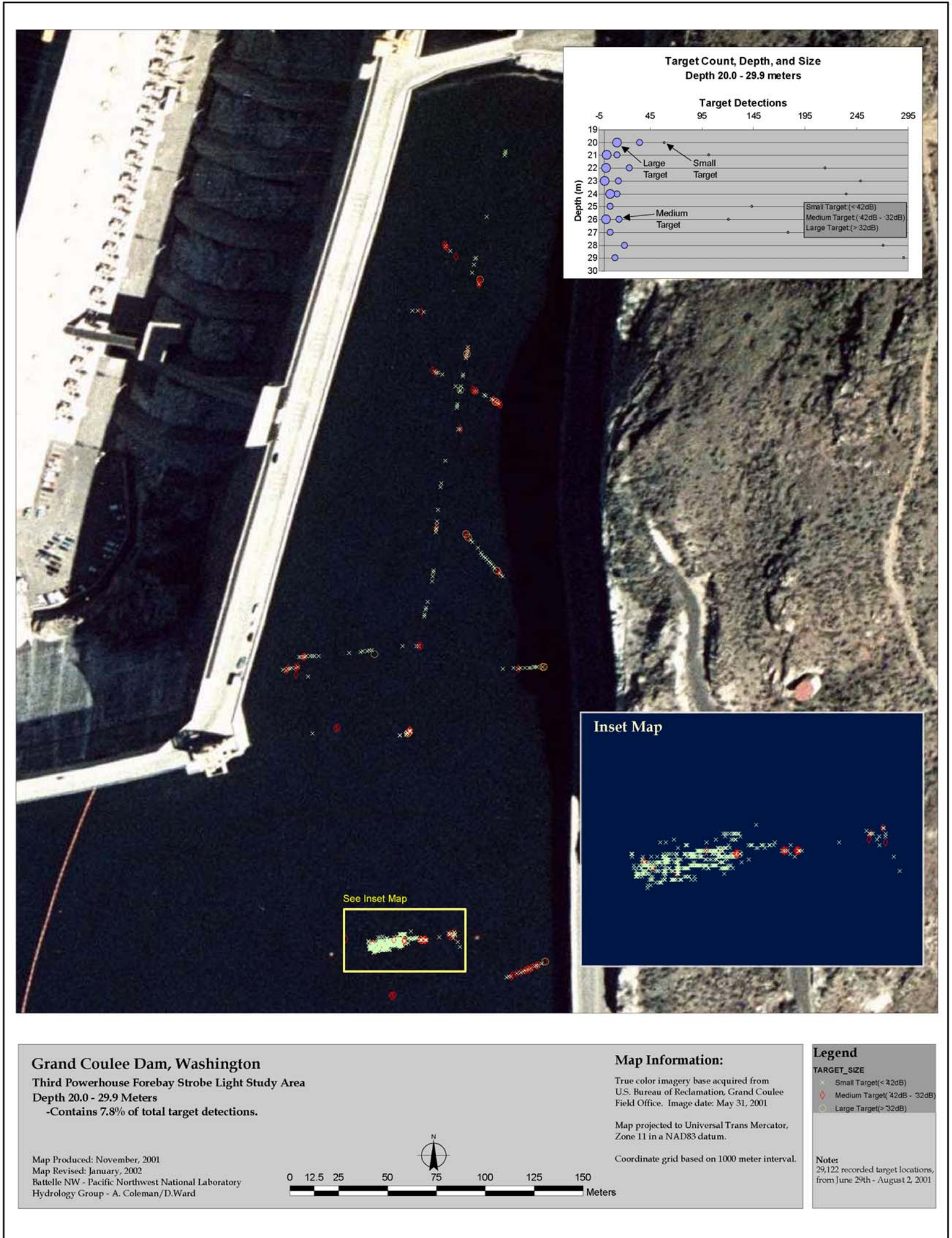
Figure B.6. Location of Targets Between 20-29.9 m from the Surface Detected by the Mobile Hydroacoustic Surveys in 2001. Three size-groups of targets are indicated based on target strength (dB).
