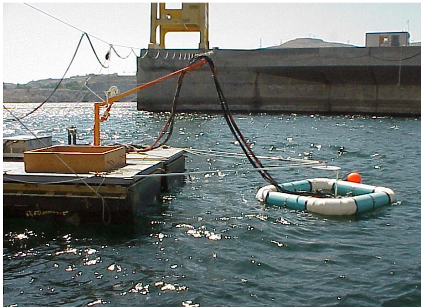
Figure E.1. Position of the Floating Calibration Frame During the Calibration Effort at Grand Coulee Dam in 2001
