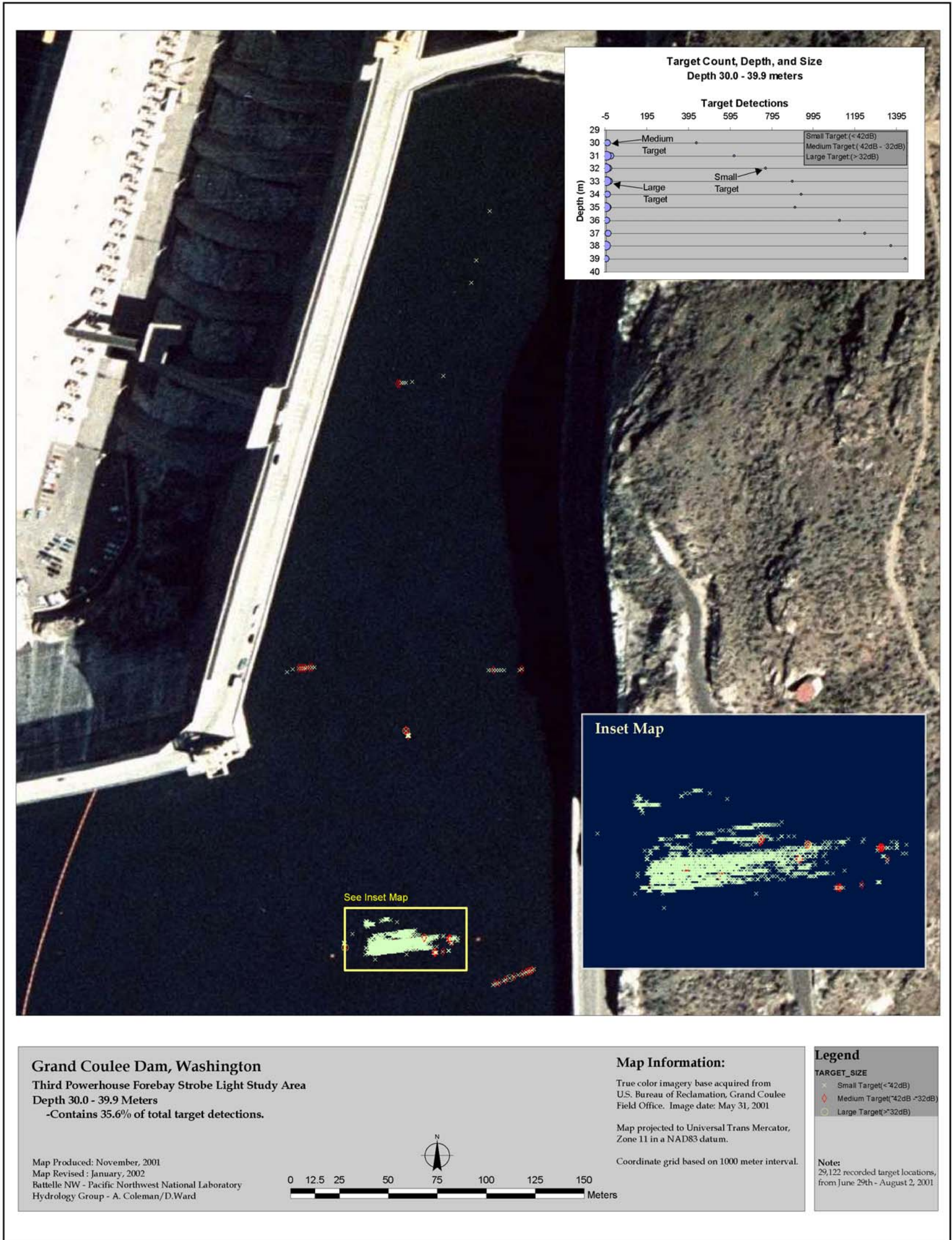
Figure B.7. Location of Targets Between 30-39.9 m from the Surface Detected by the Mobile Hydroacoustic Surveys in 2001. Three size-groups of targets are indicated based on target strength (dB).
