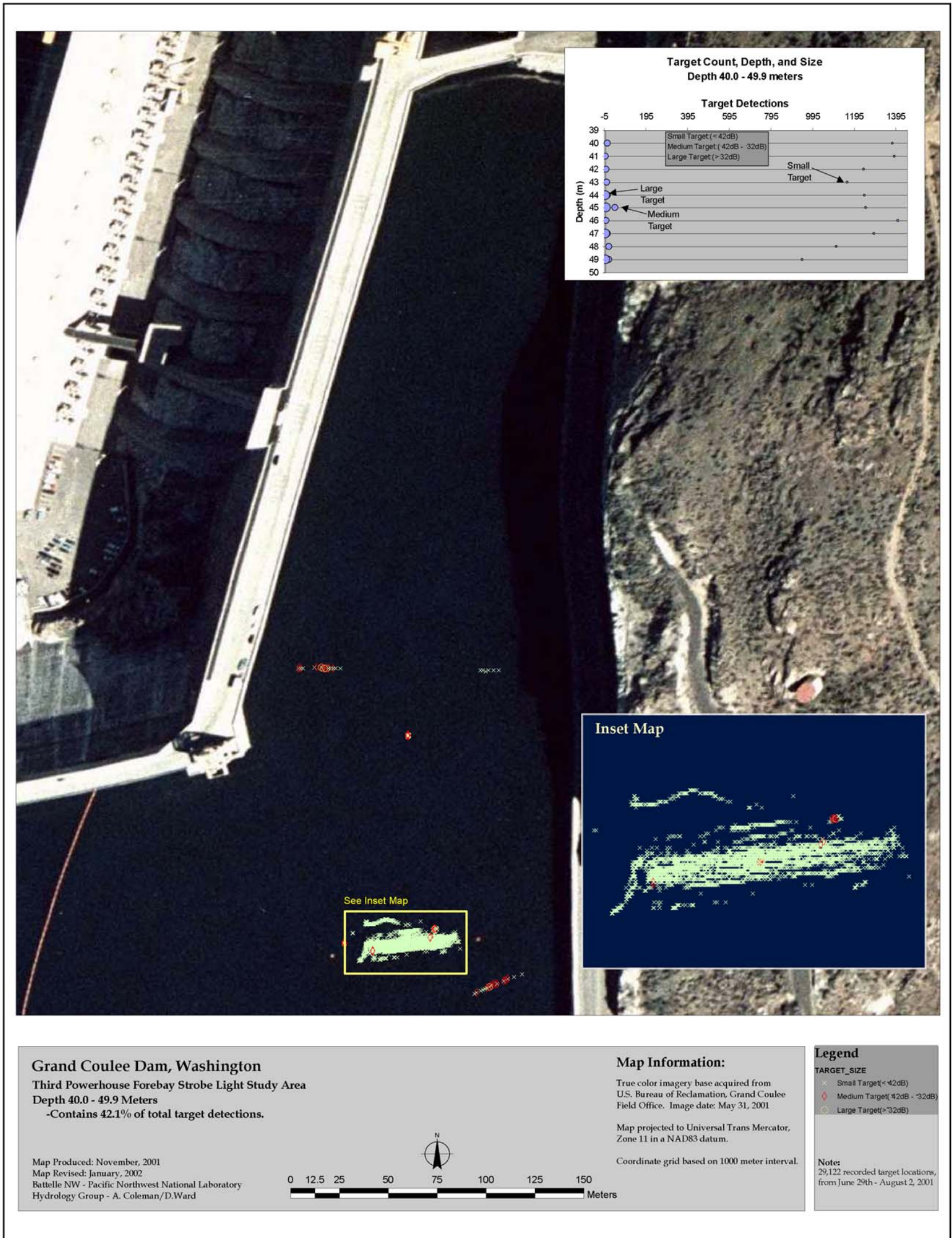
Figure B.8. Location of Targets Between 40-49.9 m from the Surface Detected by the Mobile Hydroacoustic Surveys in 2001. Three size-groups of targets are indicated based on target strength (dB).
